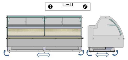
2. If the appliance is not levelled in some of its directions, remove the bottom coverings for enabling access to the adjustable feet. Check especially the central foot adjustment.
