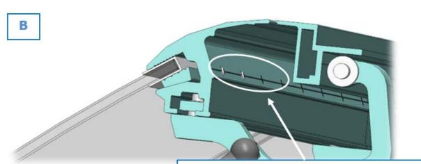
SLIGHTLY LOOSEN THE DIN913 SET SCREWS.
