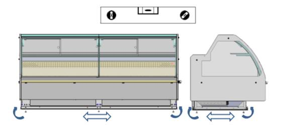
2. If the appliance is not levelled in some of its directions, remove the bottom coverings for enabling access to the adjustable feet. Check especially the central foot adjustment.
